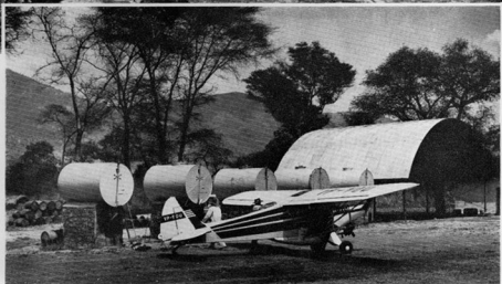
Above: Muze base camp on the edge of the Rukwa plains, showing the European staff houses at the top, the workshops in the centre and the African staff houses in the foreground. Right: The landing strip at Muze. The tanks behind the Piper Cub contain insecticide, which is about to be fed into the belly tank under the aircraft.
