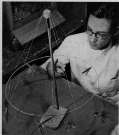
Above: Mr. Charl du Plessis, Director of the service, in his office at Abercorn. Left: Locust research is carried out not only in Central Africa, but in London as well. Here, at the Anti-Locust Research Centre, London, locusts are made to fly by suspending them from a wire frame hung from a central pivot. Feeling themselves suspended in air, the locusts begin to fly and turn the "roundabout". This gives an estimate of their speed and duration of flight. These specimens are desert locusts.
